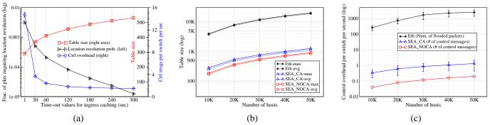
Figure 4: (a) Effect of cache timeout in AP-large with 50K hosts (b) Table size increase in DC (b) Control overhead in AP-large.
