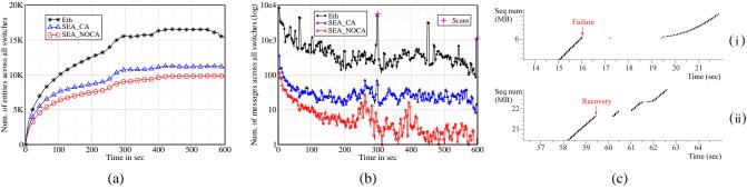
Figure 8: Effect of network dynamics: (a) table size (b) control overhead (c) failover performance.
